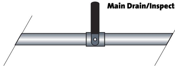
**Main Drain/Inspector Test** - this valve is used for testing the system, see the instructions on the back to do the flow test.
